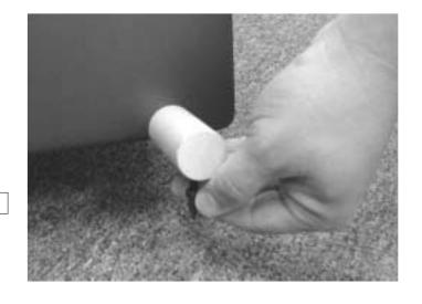
screw the metal spikes into the bottom of the aluminum stabilizer bars. Tighten the locking nuts by hand. Move to the other side and repeat the procedure.
